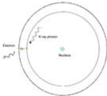
Figure 2: X-ray photons of suitable energy interact with electrons, either releasing them from the atom (ionisation) or pushing them into a higher energy orbital. In the process, the photon may be completely absorbed, or reduced in energy. The interaction may also cause deflection of the photon (see Table 2).
