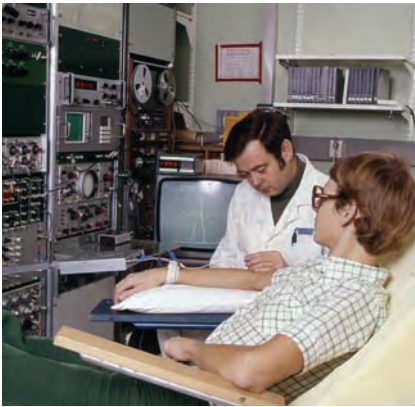
Figure 1: The author and his engineer (1977) in front of their assembled EMG recording system. Large, multi-knobbed and very flexible equipment connected to a separate computer.
