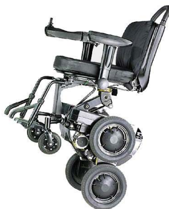
Figure 7: Gyroscopically-controlled standing wheelchair.
